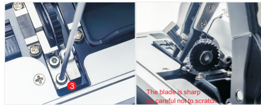
7. Use an M1.5 Allen wrench to unscrew "Screw 3" and then remove the blade holder upwards.
