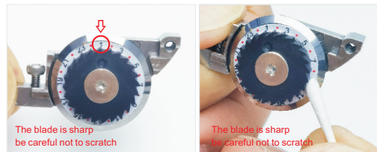
9. Confirm that the "cutting point number 1" of the new blade assembly is facing upwards, as shown in the figure. If not, use a cotton swab to rotate the blade so that number 1 is facing upwards (if the cutting point numbers do not match after installation, you can enter the "Blade Usage Details and Rotating Blade Surface" of the "Cutter Settings" of the APP to "Correct the Point").
