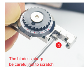
8. Use an M1.5 Allen wrench to remove "Screw 4", which needs to be installed on the new blade assembly later.
